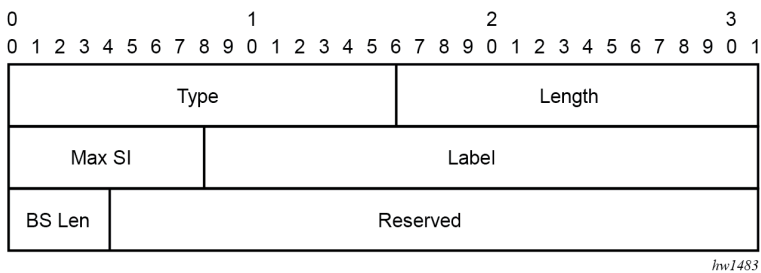
Figure 30: BIER MPLS Encapsulation sub-TLV format
