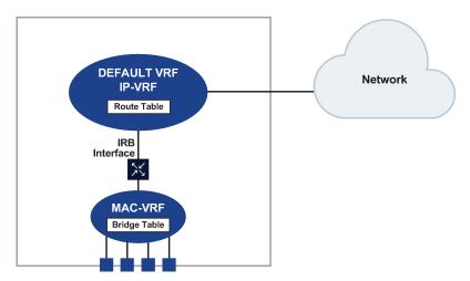
Figure 8: MAC-VRF, IRB interface, and IP-VRF
